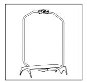
Place the frame in the weighing chamber. The wedgeshaped opening at the top of the frame must face the direction from which the sample holder (sieve/glass plummet) will be placed into the frame.
