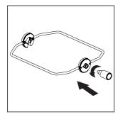
Screw the corresponding adapter into the bar frame base from below:
